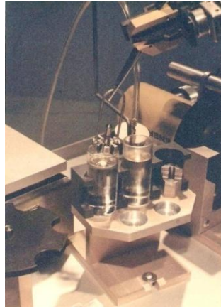
Gambar 4. Uji Kebocoran Outer Capsule
